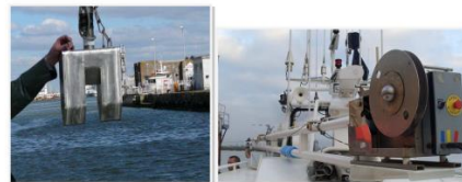
Fig. 3. X Ray profiler and winch system
